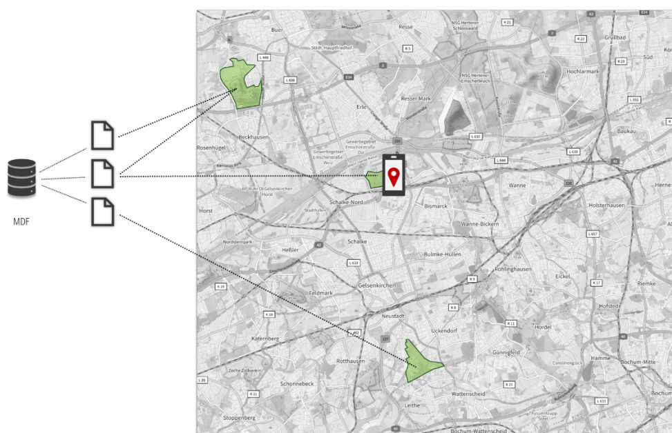
Figure 9. The principle of My Dynamic Forest (MDF) tool. An MDF instance is able to host various questionnaires (left). Any given questionnaire is typically linked (geofenced) to an area of interest, as indicated by dotted lines. Notably, a given questionnaire may be linked to a single or to multiple areas of interest, and conversely, any given area of interest may be linked to one or more questionnaires. Subsequently, if a device is located within an area of interest, available questionnaires are determined, and responses spatialised.
